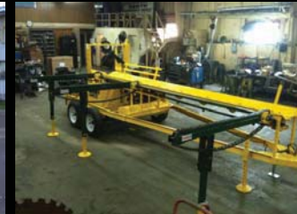
CORD KING M2030 with standard 16' infeed and 3 leg live deck
