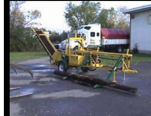
CORD KING M1418 with log lifter and integrated 12' conveyor
